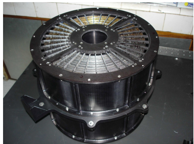
Figure 3.1: Left: Structure and various components of the Soft X-ray Telescope from outside (simulated picture). Top: The optical modules with gold-coated mirrors (upper: 1-alpha; lower: 3-alpha; actual photo).
